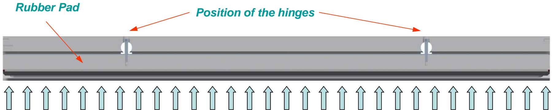
*Self adjustment means constant application of load from the rubber pad to the blanket cylinder*
